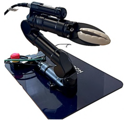
Fig. 1: Reach Alpha 5, a 5DoF underwater manipulator arm equipped with a mounted camera used in our experiments.
