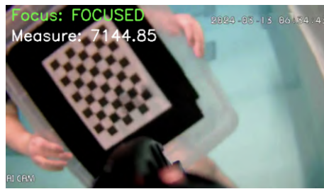
(b) A sample frame where the checkerboard is in focus.
