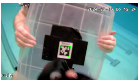
(a) A 50mm AprilTag at 0.44m, the farthest distance before it becomes undetectable.
