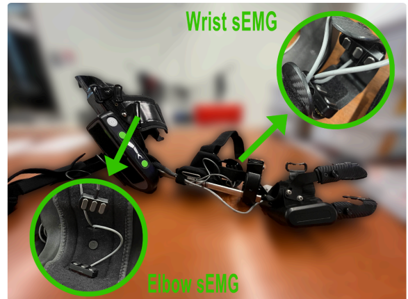
Fig. 1: Overview of the MyoPro 2 device, highlighting the placement of sEMG sensors.
